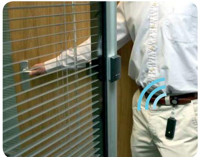
Our hands free interface is simply installed between the reader and the Intelligent Control Unit
